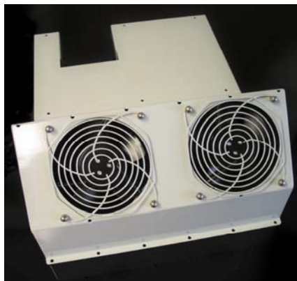
Figure 9 - Fan shroud removed from ELSAT ® BUC
