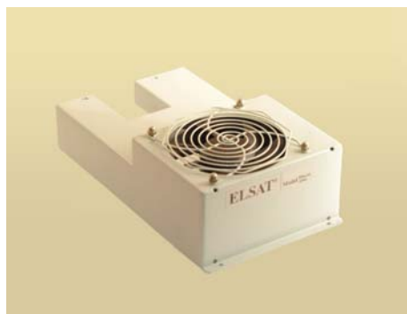
Figure 11 - Fan shroud removed from Baby BUC
